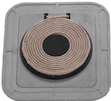
Figure D-1: Transmitter top surface
