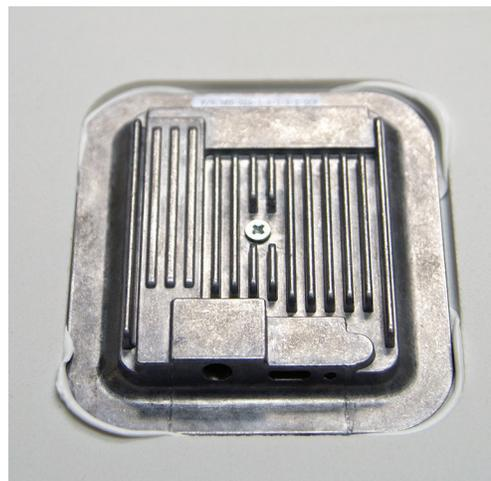
Figure D-3: Transmitter adhered to surface
