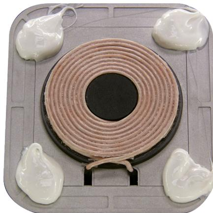
Figure D-2: 100% Silicone applied to transmitter
